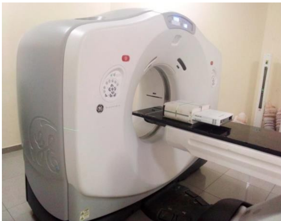
Figure 1: CT scanning of the miniPhantom with the MatriXX 2D array detector embedded in it
