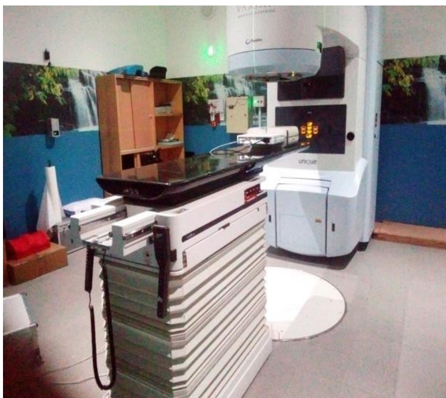
Figure 4: Treatment delivery with the miniPhantom having the MatriXX detector inserted into the phantom
