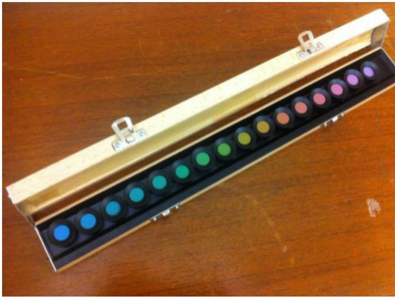
Figure 1.1: Farnsworth D-15 hue test set with 15 coloured caps with a natural hue progression
