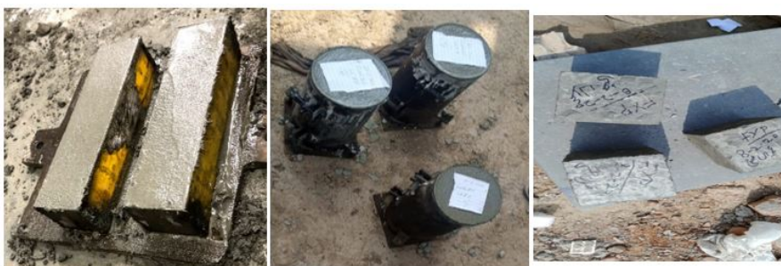
Figure 3: Casting of concrete cylinders, cubes and mortar bars
