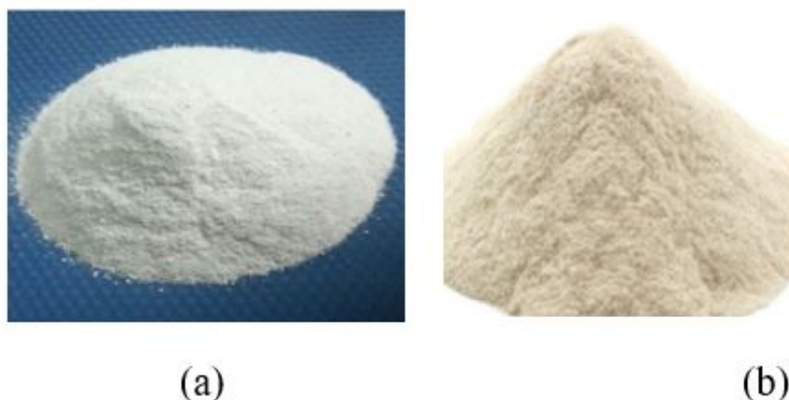
Figure 1: Cementitious material: (a) Glass Powder(SSG), (b) Xanthan Gum
