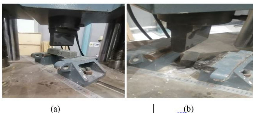
Figure 7: Experimental setup: (a) Sample (mortar bar) before testing & (b) after testing
