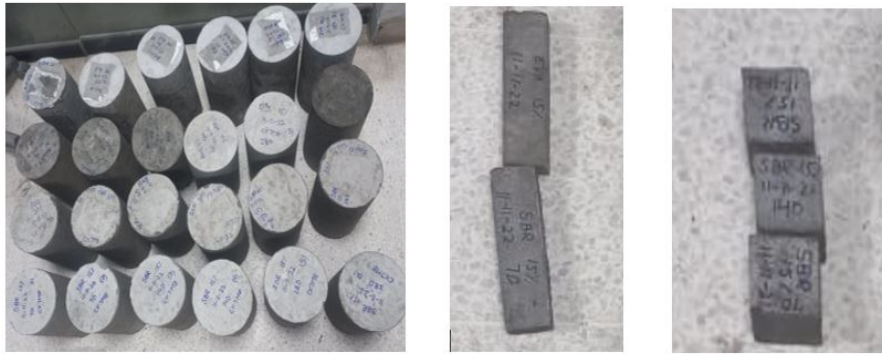
Figure 4: After casting hardened concrete cylinders, cubes and mortar bars
