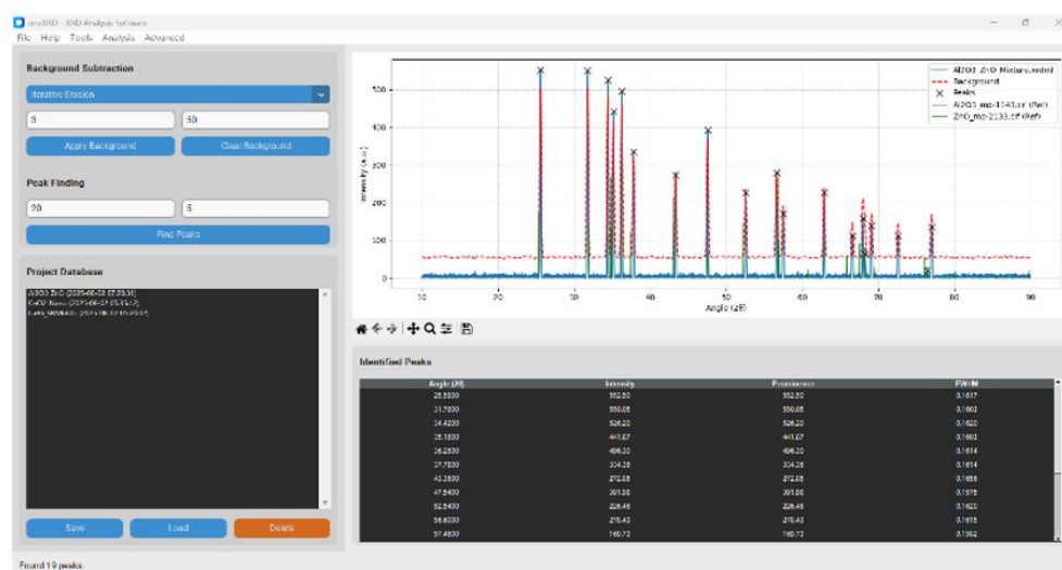
Figure 12: The oneXRD main window showing the fully prepared analysis. The experimental data from the mixture is plotted, the background is subtracted, peaks are found, and the two reference patterns for \text{Al}_2\text{O}_3 and \text{ZnO} are overlaid.
