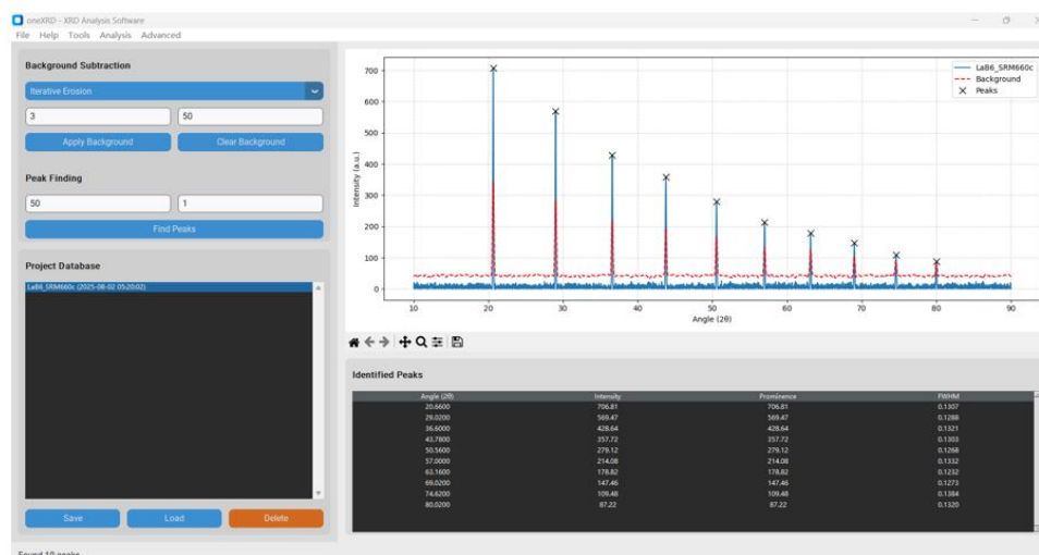
Figure 8: Processed XRD pattern of NIST SRM 660c (LaB 6 ) in oneXRD. The plot displays the raw experimental data, the calculated background (red dashed line) after iterative erosion, and the automatically identified peaks (black 'x' markers).
