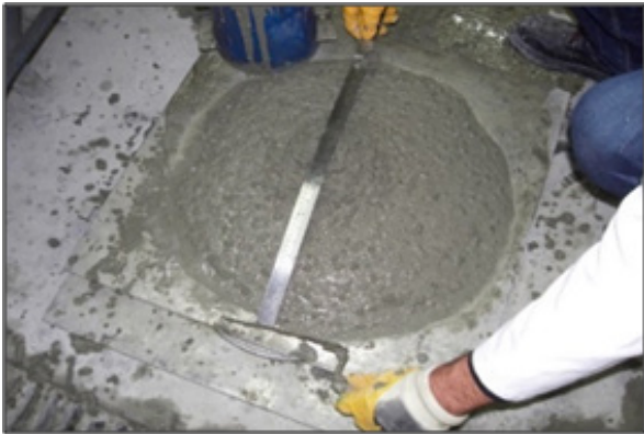
Figure 10. Flow diameter measurement of SCC
