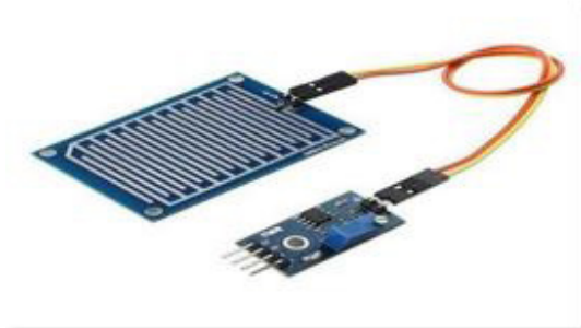
Figure 5: Rain Sensor Module
